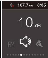
Scroll (Button 3) until you see the interface (left). Once here, press (Button 3) to enter the volume mode. Scroll up or down to change the volume.
