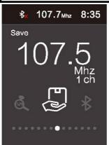
Scroll (Button 3) until you see the interface (left). Once here, press (Button 3) and it will save the current radio station you are listening to. You can save up to 10 stations on this device.
