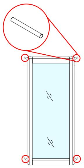
**Part 2:** When the door is placed into position between the left and right glass frames, the spacer and nut will secure the metal rod. The spacer and nut is screwed inside the left and right glass frames as shown below. Use the pre-made hole to reach the metal rod.
