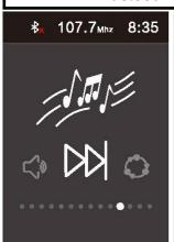
To change track whilst in the sauna form the panel, scroll to the audio interface (left). Then press the scroll (Button 3) and it will change to the next track. This will also change through the saved radio station list you have made. You can only skip forwards, not backwards.
