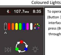
To operate the lights, press (Button 3) until you see the interface (left). Once here press (Button 3) and scroll through the light options.
