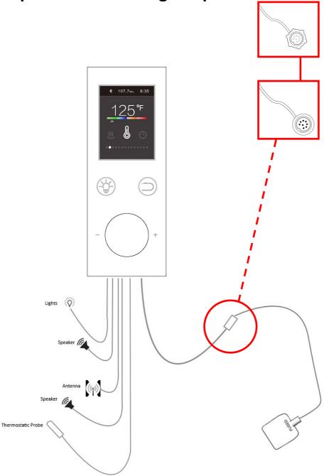
**Part 1:** Connect the control panel to the lights and speakers, located in the roof.
