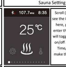
Scroll (Button 3) until you see the interface (left). Once here, press (Button 3) to enter the sauna mode. This will toggle the Sauna heater on/off as desired. Use the Time/Temp settings to make the most out of your session.
