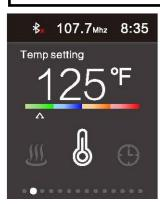
For temperature: Scroll (Button 3) until you see the interface (left). Once here, press (Button 3) to enter the temp mode.
