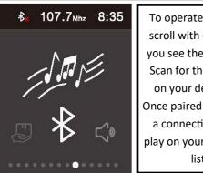
To operate the Bluetooth, scroll with (Button 3) until you see the interface (left). Scan for the control panel on your device and pair. Once paired you should hear a connection tone. Press play on your device to begin listening.
