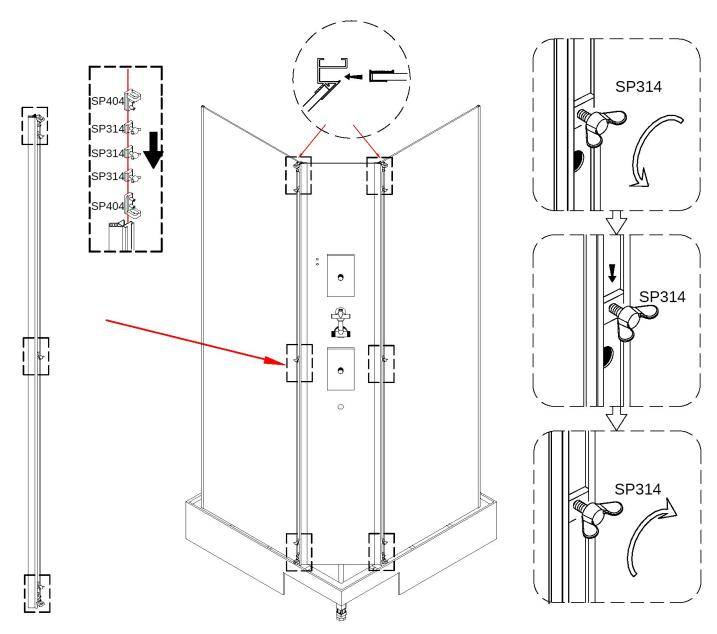
**Step 5** — **Installing the Upright Profiles**
